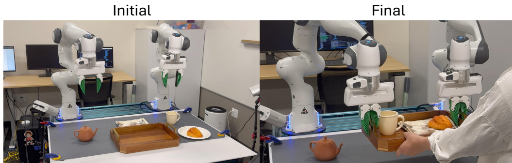
Figure 9: Initial configuration and successful final configuration of the preparing breakfast tray task.
